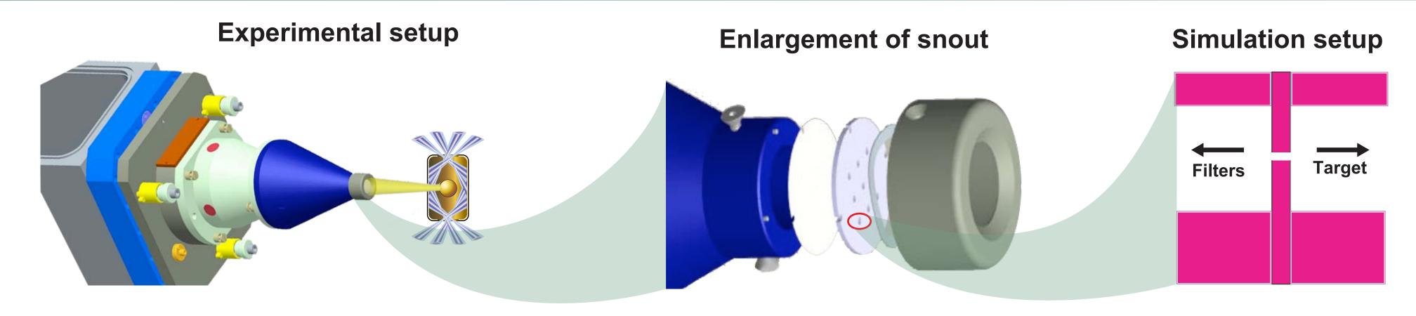
Requirements on shrapnel size and velocity depend on filter material and thickness
