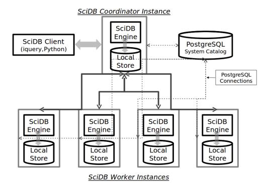
SciDB is deployed on a cluster of servers, each with processing, memory, and local storage, interconnected using a standard ethernet and TCP/IP network. Each physical server hosts a SciDB instance that is responsible for local storage and processing.
