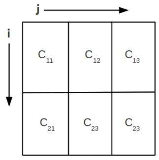
Chunks are arranged in row-major order in this example, and stored within the cluster using a round-robin distribution as follows. Suppose a cluster has instances 1 through 4, the placement of data is shown below.
