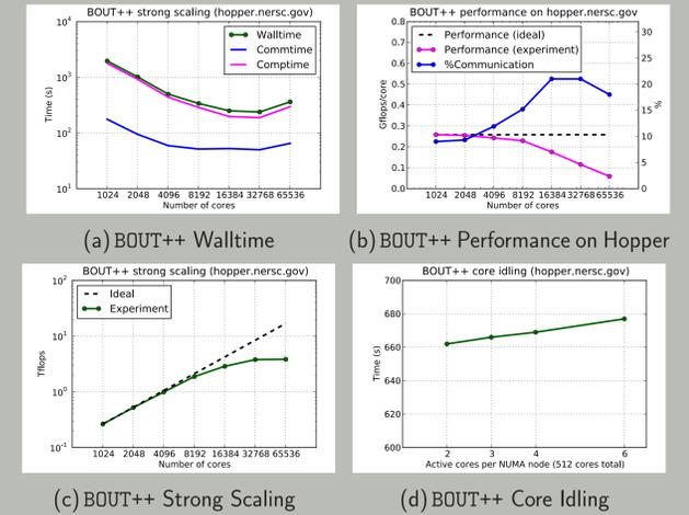
Figure 1: Strong scaling using CrayPAT on Hopper (NERSC) using ELM\_pb (nx=516, ny=512, nz=64) [2]
