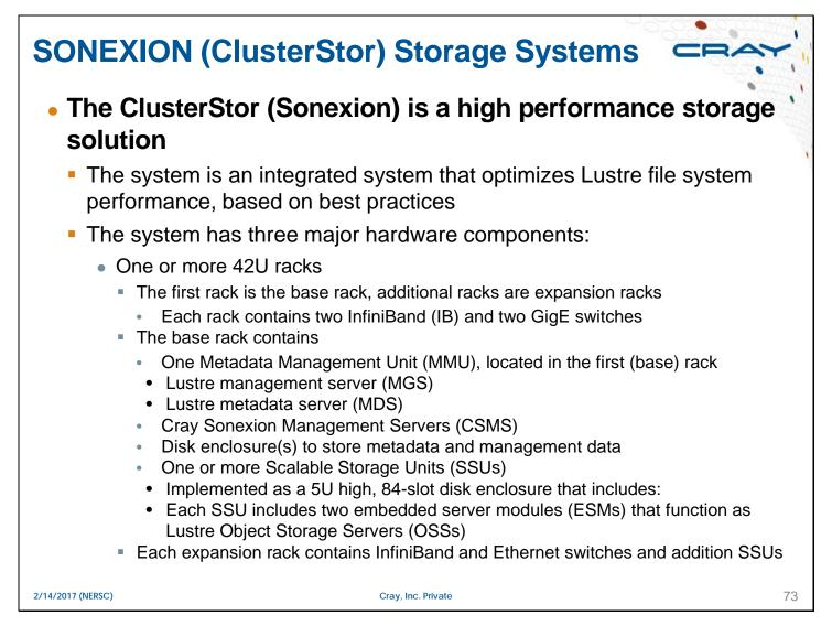
Each SSU contains eight logical storage devices referred to as Object Storage Targets (OSTs) and two Object Storage Servers (OSSs) that provide file I/O service and network request handling for the client(s). Each OST is a RAID6 (8+2) array of disk drives. The SSU also contains two global hot spares and a mirrored pair of SSDs to store Journaling information.
