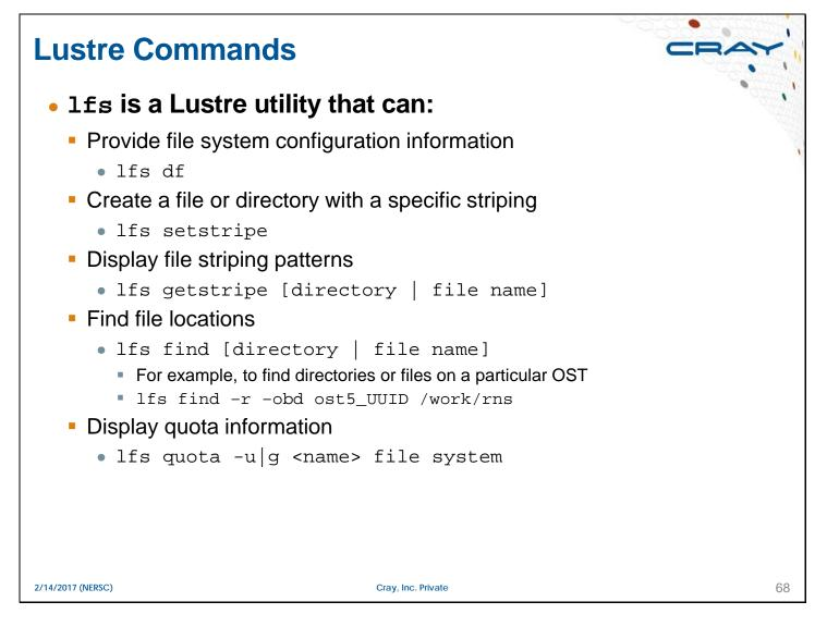
The stripe utility, lfs, enables you to stripe files after Lustre is configured. Normally, you stripe files by using the lmc command when you create the configuration file.
