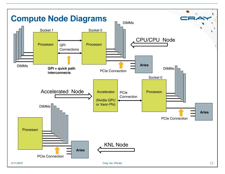
The QPI (quick path interconnect) link operates at approximately 6.4 GT/s or 25.6 GB/s. The two socket configuration provides a peak bandwidth of 51.2 GB/s.
