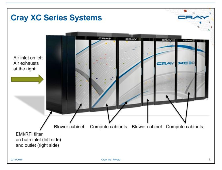
Single air inlet (left side) and exhaust (right side) per row. An optional preconditioning coil (located on inlet side of the first blower cabinet in each row) relaxes inlet air requirements. The exhaust air is conditioned (cooled) air. The exhaust air can be room neutral depending on the environmental conditions.
