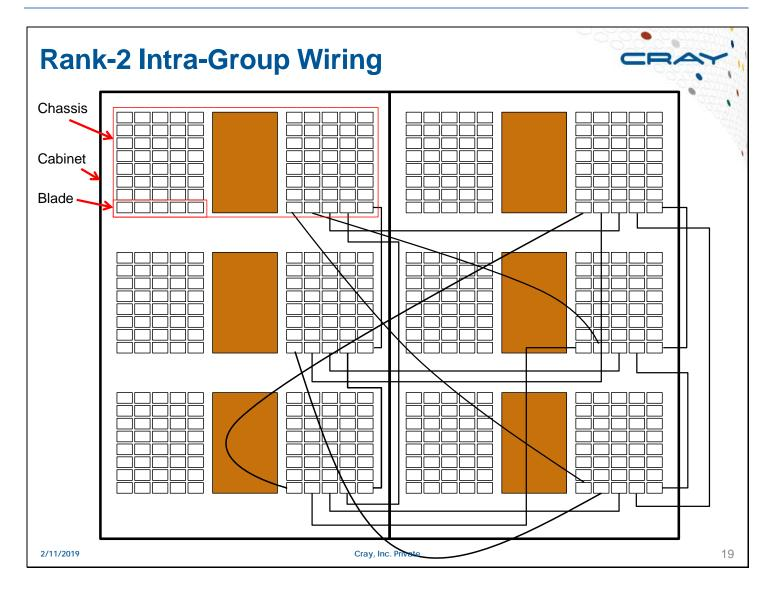
This slide shows the electrical cable connections between slot 0 in all 6 chassis for a two-cabinet group. This cabling pattern is repeated for the other 15 slots in each chassis.
