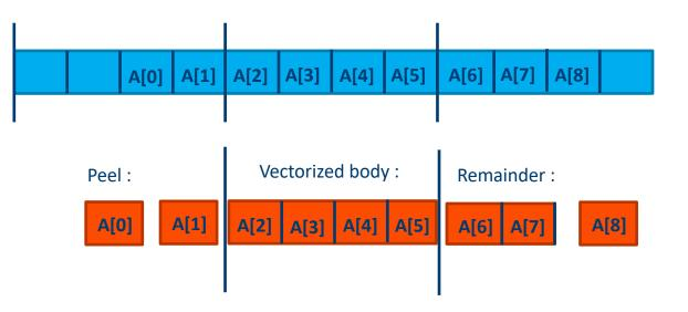
Compiler can split loop in 3 parts to have aligned access in the loop body
