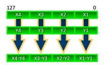
**SSE** Vector size: **128 bit** Data types: 8, 16, 32, 64 bit integer 32 and 64 bit float VL: 2, 4, 8, 16
