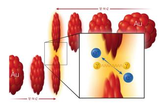
Making matter from light: Two gold (Au) ions (red) move in opposite direction at 99.995% of the speed of light (v, for velocity, = approximately c, the speed of light). As the ions pass one another without colliding, two photons ( $\gamma$ ) from the electromagnetic cloud surrounding the ions can interact with each other to create a matter-antimatter pair: an electron (e-) and positron (e+). Image: Brookhaven National Laboratory
