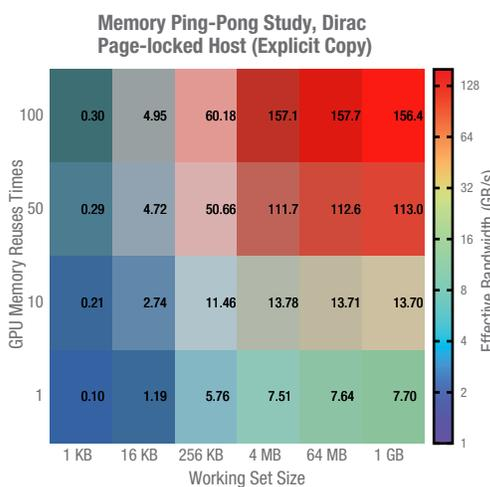
(b) Page-locked host with explicit copy between CPU and GPU
