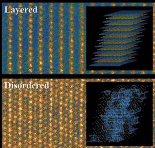
◀ Conventional layered lithium and transition metal cathode material (top) and the new disordered material studied by researchers at Massachusetts Institute of Technology (bottom) as seen through a scanning transmission electron microscope. Inset images show diagrams of the different structures in these materials. (In the disordered material, the blue lines show the pathways that allow lithium ions to traverse the material.) *Image: Massachusetts Institute of Technology*
