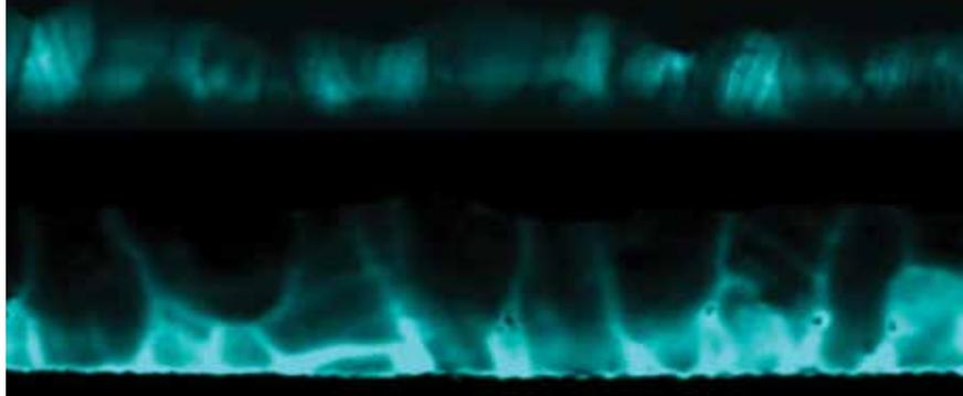
◀ Cross-sectional electron beam-induced current maps show the difference in cadmium telluride solar cells before (top) and after (bottom) cadmium chloride treatment. The increased brightness after treatment indicates higher current collection at the grain boundaries. *Image: Chen Li, Oak Ridge National Laboratory*
