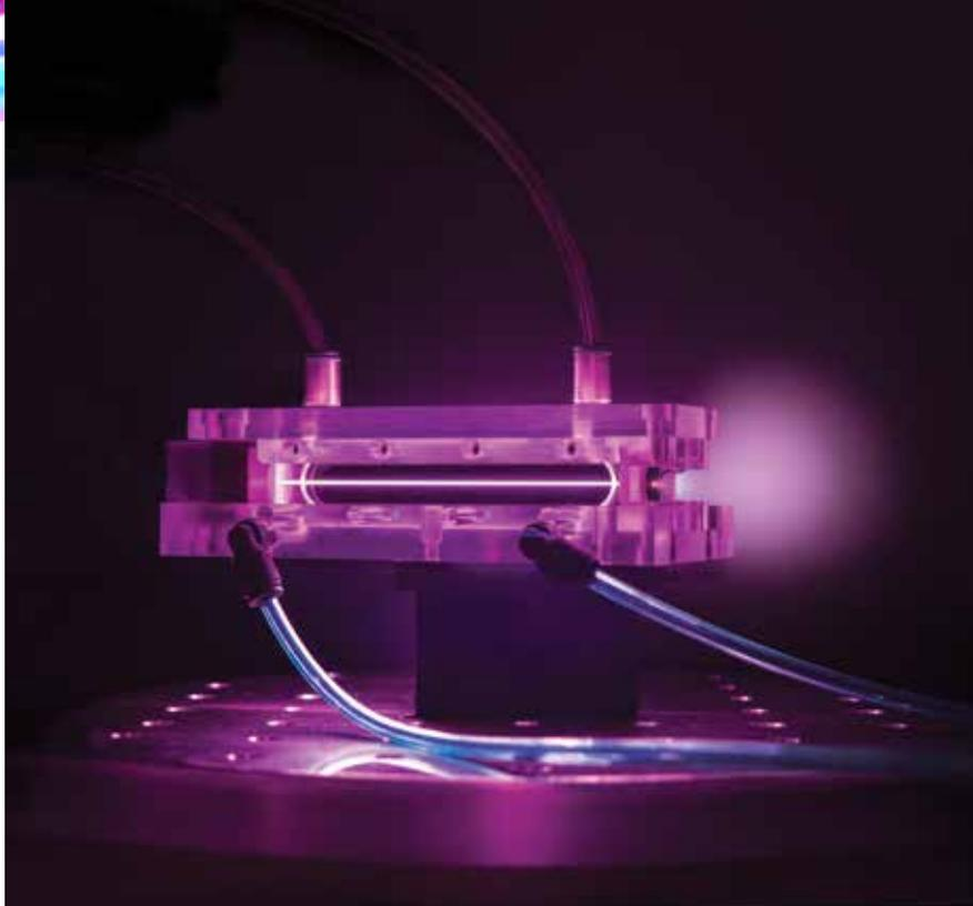
◀ A 9 cm-long capillary discharge waveguide was used in BELLA experiments to generate multi-GeV electron beams. The plasma plume has been made more prominent with the use of HDR photography. Image: Roy Kaltschmidt, Lawrence Berkeley National Laboratory
