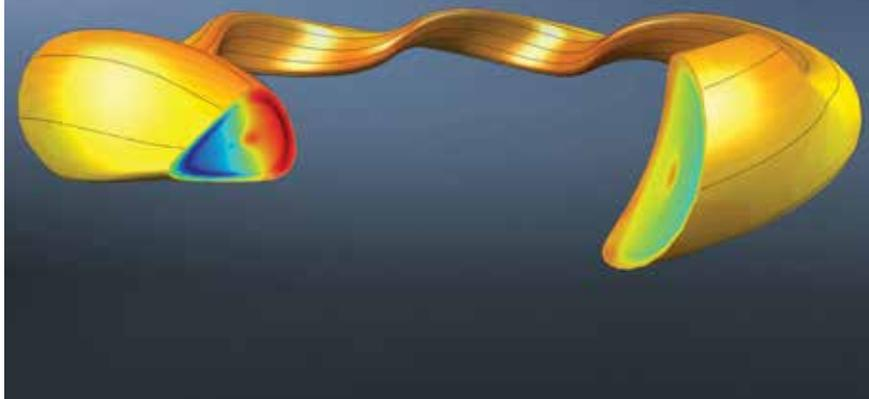
◀ A calculation of the self-generated plasma current in the W7-X reactor, performed using the SFINCS code on Edison. The colors represent the amount of electric current along the magnetic field; the black lines show magnetic field lines. Image: Matt Landreman, University of Maryland
