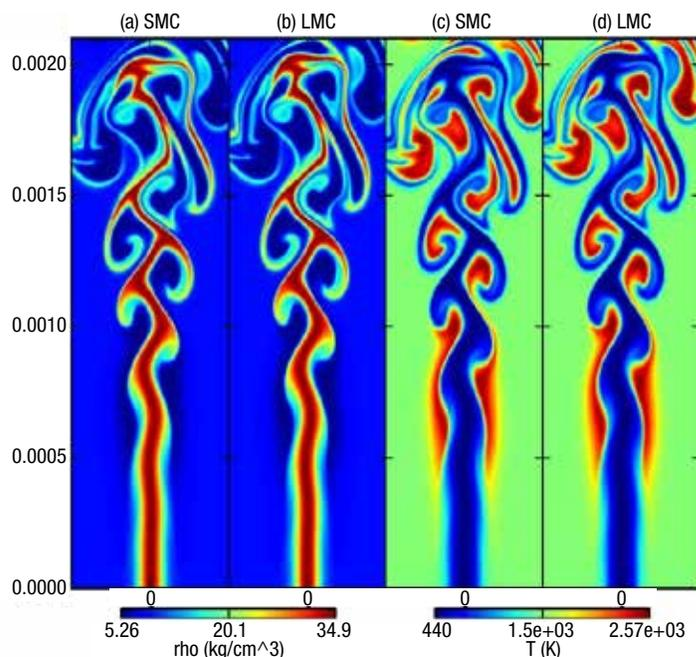
◀ This simulation illustrates the total mass density (left) and temperature (right) of a dimethyl ether jet fuel simulation. It is a snapshot of the solution that corresponds to a physical time of 0.00006 seconds. *Image: Matthew Emmett, Weiqun Zhang, Lawrence Berkeley National Laboratory*
