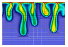
A snapshot of CO<sub>2</sub> concentration after onset of convection showing an AMR grid with 3 levels of refinement.
