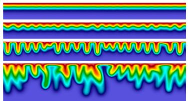
Density of aqueous CO<sub>2</sub> as a function of time (increasing from top to bottom).
