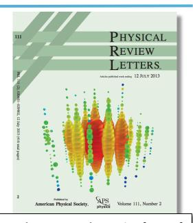
On the Cover: Schematic of one of the two PeV-energy neutrino events detected by the IceCube detector. Each sphere represents a detector sensor. Sphere size is a measure of detector response. Colors represent arrival times (red, early; blue, late). These two events could be the first ever hints of neutrinos from astrophysical sources.
