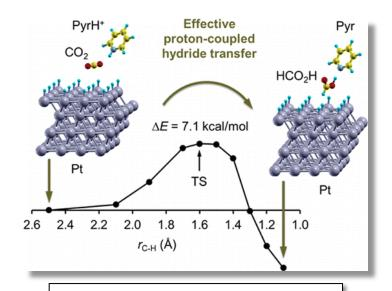
Results of electronic structure computations done at NERSC explaining the precise mechanism of a reaction in which CO<sub>2</sub> is converted to formic acid (HCO<sub>2</sub>H, an important intermediate in chemical synthesis) using platinum (Pt)
