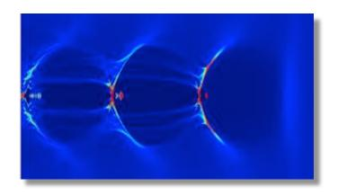
Simulation of a laser plasma wakefield as it evolves in a 9-cm long tube of plasma. The charge "wake" (three are shown) allows electrons to "ride" the wake to greater and greater speeds and energies. The work was selected as one of ten Best Physics Papers of 2014 by Scientific American.
