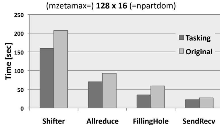
Performance breakdown of GTS shifter routine using 4 OpenMP threads per MPI process with varying domain decomposition and particles per cell.
