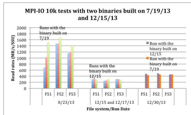
Figure 6. This figure shows the MPI-IO 10k read rates (read-after-write) measured by the two binaries that were built for the August acceptance tests (built on 7/19) and for the December retest (built on 12/15/13).
