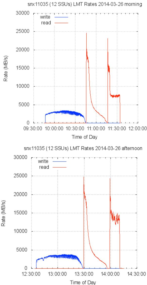
Figure 10. The LMT data for the two MPI-IO 10k jobs ran on 3/26/2014 (the same two jobs as in Fig. 8). The second read curve in each panel is the read rate from the re-read job.
