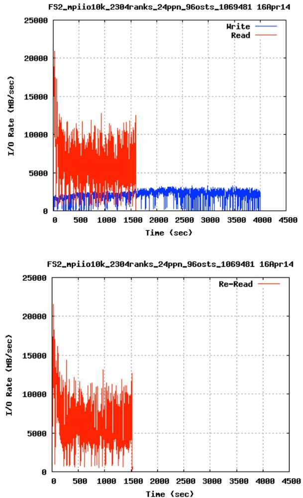
Figure 16. The figure shows the I/O rates for an MPI-IO 10k standard test (write and then read, upper panel), and a re-read test (lower panel) on FS2. These tests were run under the production environment. Between the write and read phases during the standard run, the compute node kernel and Lustre caches were cleaned up.
