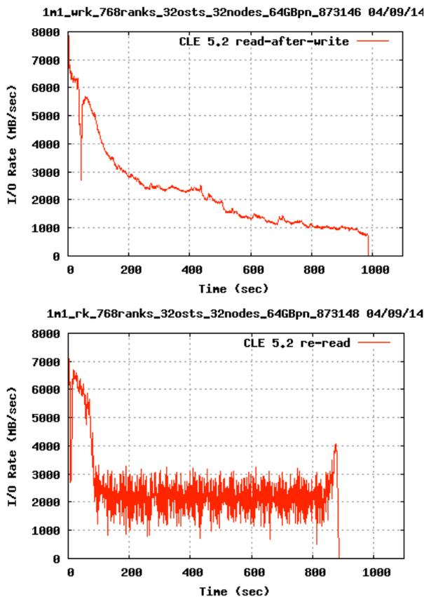
Figure 7. The distinctive read profiles for the read-after-write (upper plot, write rates are not shown) and the re-read test (lower plot) observed on the internal Cray R&D XC30 system with dual socket 12-core Ivy Bridge processors with 64 GB per node memory (dedicated). 32 nodes, 32 OSTs and 64GB/node file size were used in the tests. Instead of the MPI-IO 10k test, the equivalent MPI-IO 1m1 test without collective buffering was run in the tests.
