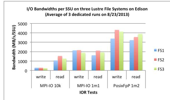
Figure 2. (a) The bandwidth per SSU obtained with three selected IOR benchmark tests with both Posix file per process and MPI-IO shared file tests on the three Lustre file systems on Edison.
