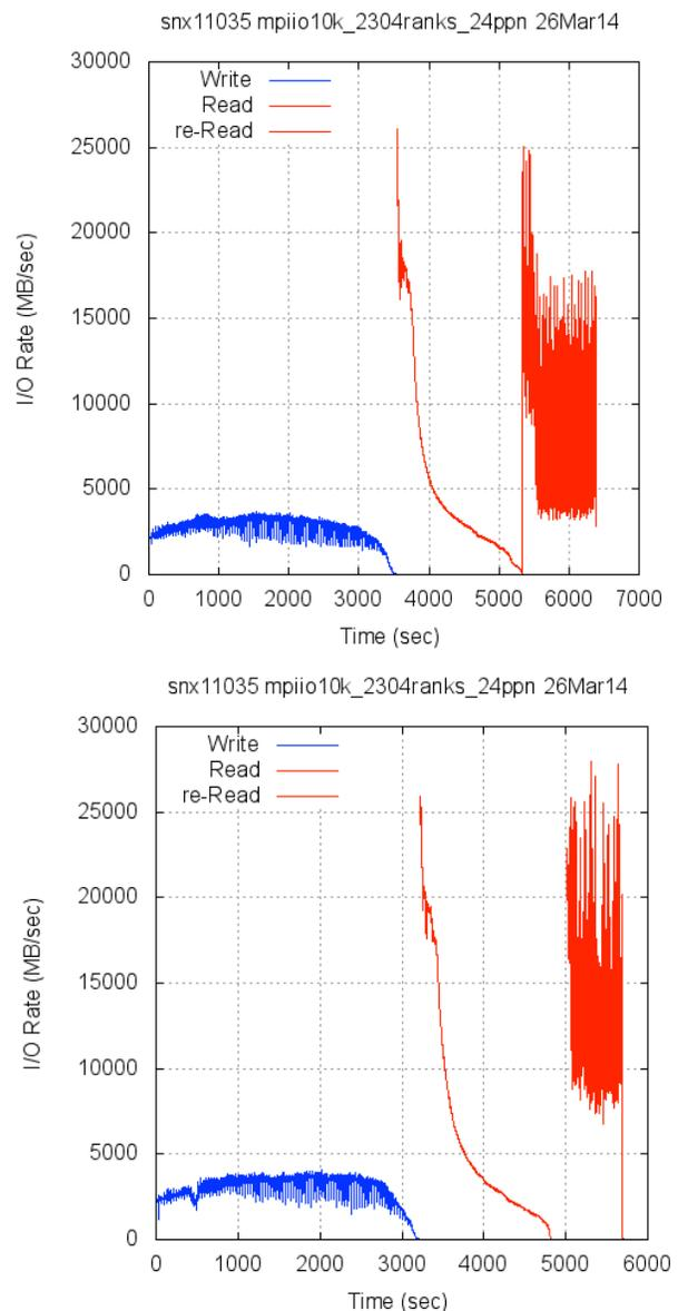
Figure 8. The I/O rates measured by the instrumented IOR for the two MPI-IO 10k jobs that were run on Edison FS2 in dedicated mode on 3/26/2014. The second read curve shows the read rate from the re-read job.
