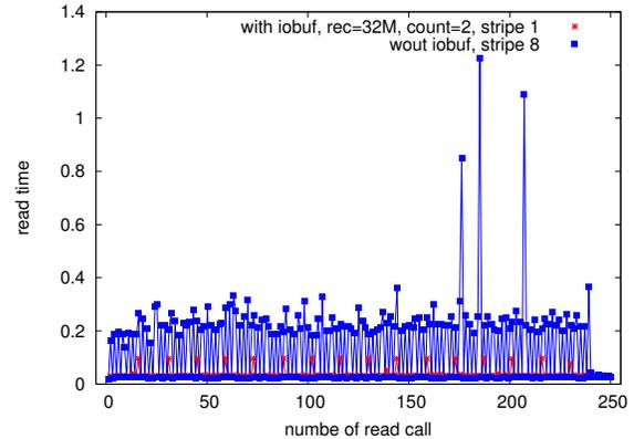
Figure 17. File read time comparison of a user code, Q LUA [11], with and without using the IOBUF library. The stripe count was also changed from the default 8 to 1. This figure was provided by a NERSC user.
