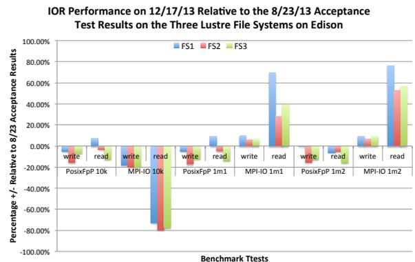
Figure 4. The IOR performance tests on December 17, 2013 on dedicated Edison system. The performance data was shown is relative to the last August results.
