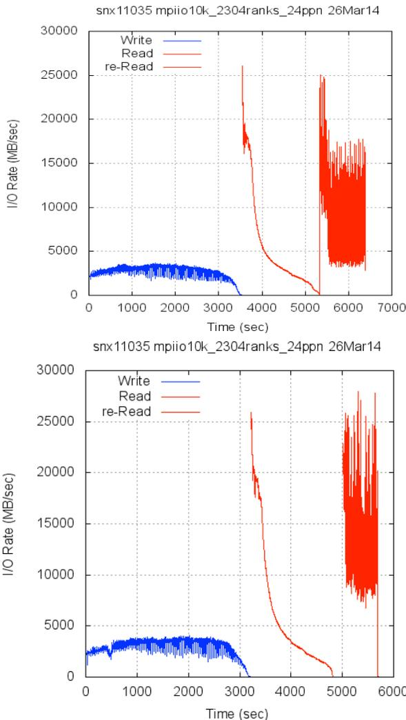
Figure 15. Dedicated MPI-IO 10k test runs on FS2 with the `readcache_max_filesize` of 1MB (upper panel, the current value) and “infinite” (lower panel, the value in August, 2013). The IOR rates were from instrumented IOR.
