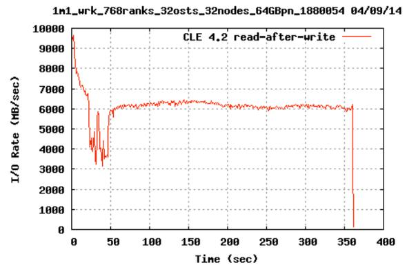
Figure 14. The read rates measured by the instrumented IOR for an MPI-IO 1m1 test without collective buffering under the CLE 4.2 and Lustre client 1.8.6 on the internal Cray R&D Cray XC30 system.
