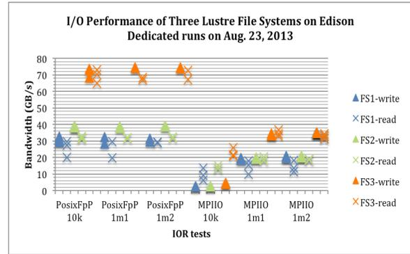
Figure 1. The IOR performance results observed in August 2013 on Edison's three file systems. Solid triangles and x's denote the write and read rates. The blue, green and orange symbols are for FS1, FS2, and FS3, respectively.
