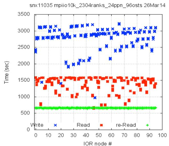
Figure 12. The write and read time per compute node. This was a dedicated run on FS2 on 3/26/2014.
