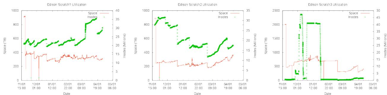
Figure 3. This figure shows the Lustre file system usage on Edison. The third file system has a larger average file size compared to the first two file systems.
