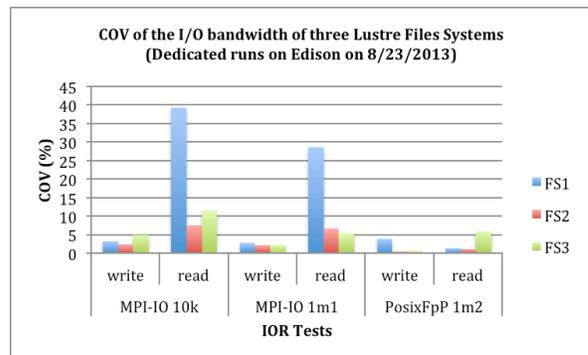
Figure 2. (b) The Coefficient of Variation (COV) of the read and write rates for the three selected IOR benchmark tests.
