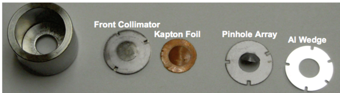
Figure 4 The front collimator, Kapton foil, pinhole array, and Al wedge placed inside GXD nose cone for a shot with nose cone 8 cm from TCC located on an equatorial position exposed to debris wind from target.
