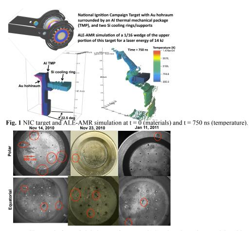
Fig. 2 Collimators in front of pinhole array for 3 re-emit shots in polar and equatorial positions.
