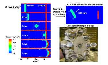
Fig. 3 ALE-AMR simulation of initial and redesigned configuration along with sample holder.
