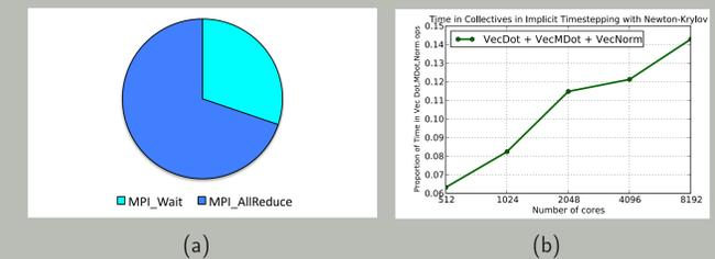
Figure 2: MPI Collectives on Hopper (NERSC)
