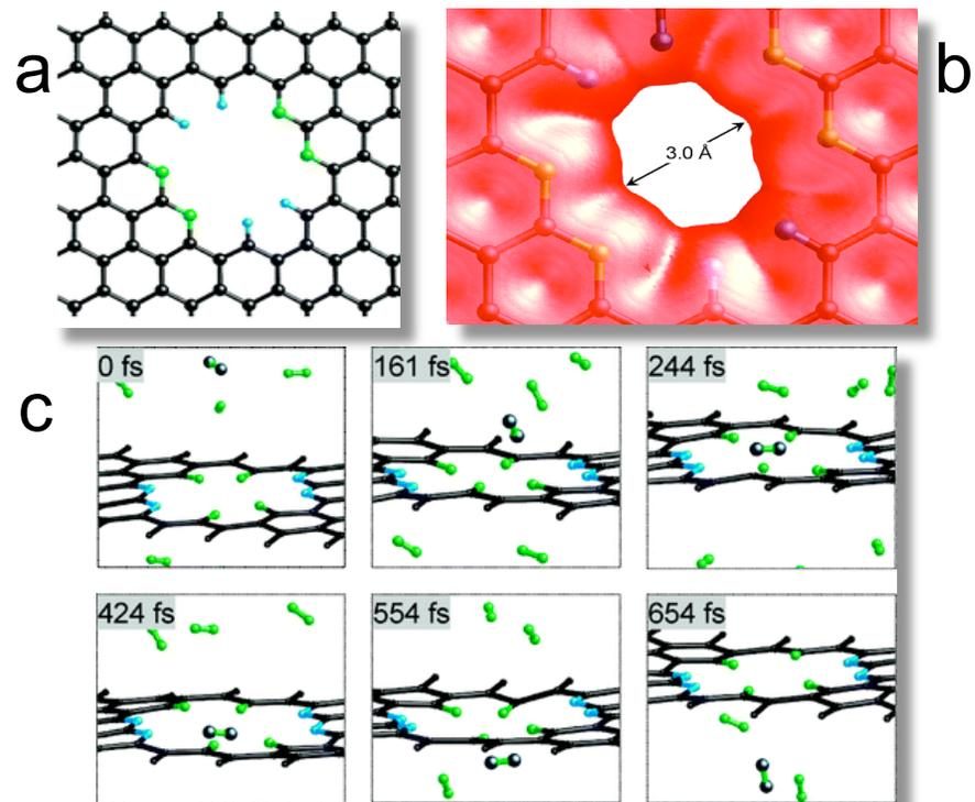
Nitrogen-functionalized pore in graphene (a), electron density isosurface (b), and snapshots of H<sub>2</sub> diffusing through the pore from NERSC first principles molecular dynamics simulations.
