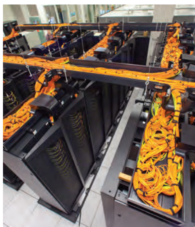
Figure 2. Top view of the Carver and Magellan clusters showing trays of InfiniBand cables. Photo: Roy Kaltschmidt, Berkeley Lab Public Affairs.
