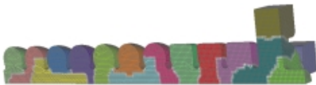
Tau3P simulation of the Next Linear Collider (NLC) Rounded Damped Detuned Structure (RDDS) output end, modeled on NERSC's T3E.
