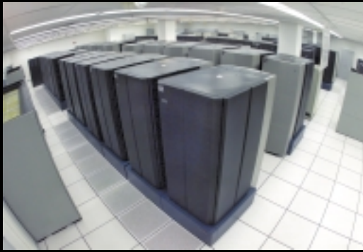
Phase 1 of NERSC's IBM RS/6000 SP system, with 512 processors and a peak performance of 410 gigaflop/s, will be replaced by the 3 teraflop/s Phase 2 system early in 2001.
